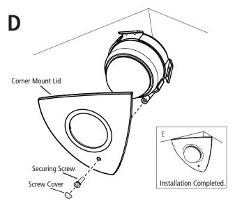
Cover the dome camera with the corner mount lid. Insert and tighten the securing screw to fix the lid to the corner mount. Insert the white screw cover to complete the installation.
